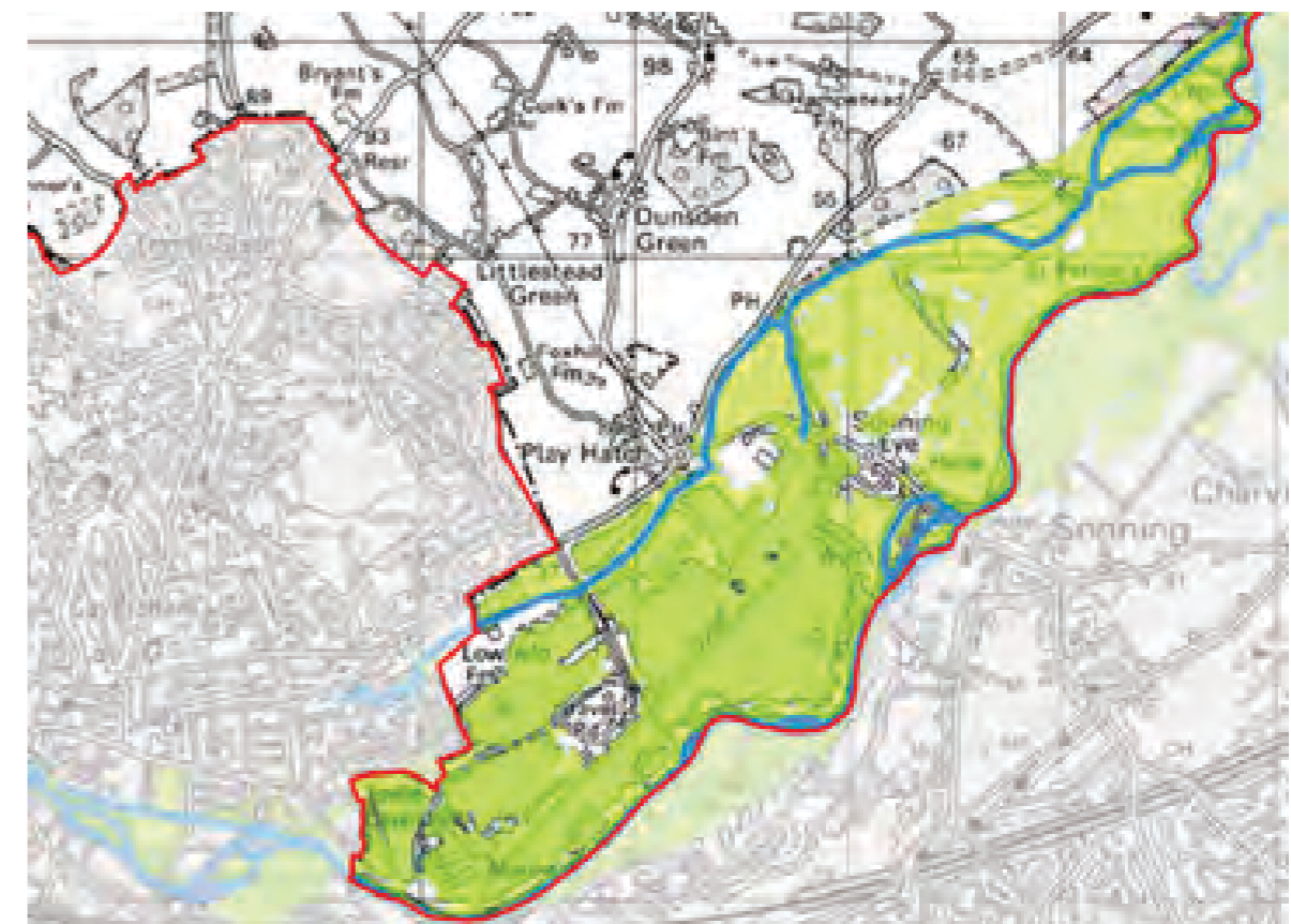
Strategic Flood Risk Assessment Map 3.1: Flood Zone 3B: The Functional Flood Plain (SODC)
